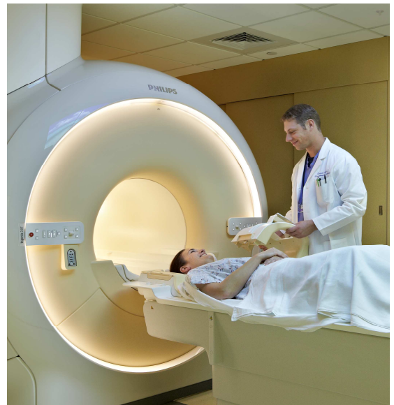
An MRI unit uses radio waves and a strong magnet to create detailed images.
