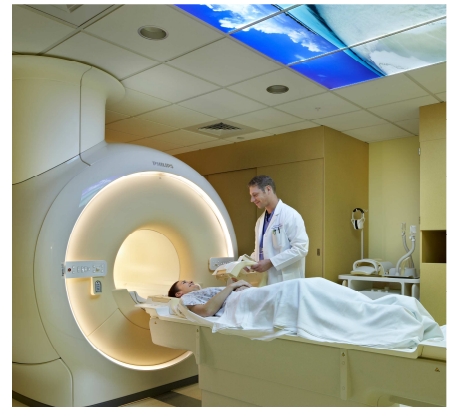
An MRI scanner uses radio waves and a strong magnetic field to create sharp images.
